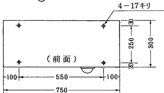
[アンカーボルト取付寸法図] (Anchor bolt mounting dimension diagram)
